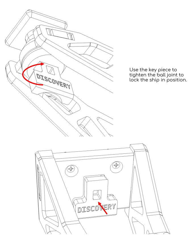
House the key piece in the wall stretcher for future use. For the first few weeks you will need to periodically tighten the ball joint to maintain the tightness of the joint.
