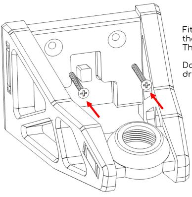
Fit the wall plugs into your wall using the spacing of the two mount points. Then Install the wall screws.
