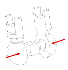
Feed the ball joint through the lower stretcher and screw the ball joint cap on to secure it in place.
