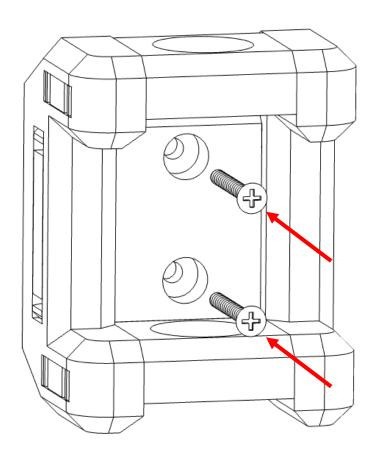
Be sure to align the holes vertically using a spirit level. Tighten the screws using a screwdriver only. Do not over tighten the screws.
