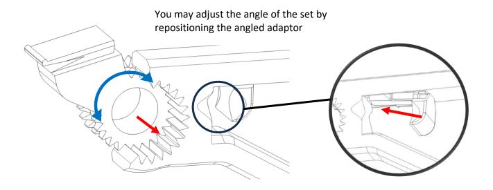
Lock the adaptor in place with the sliding clip
