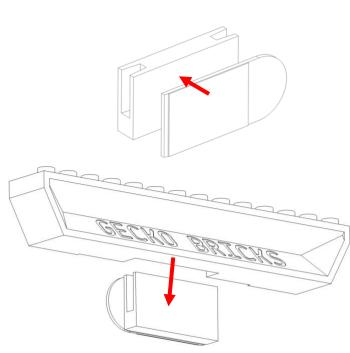
Attach the Minifigure mount lug to the wall first
