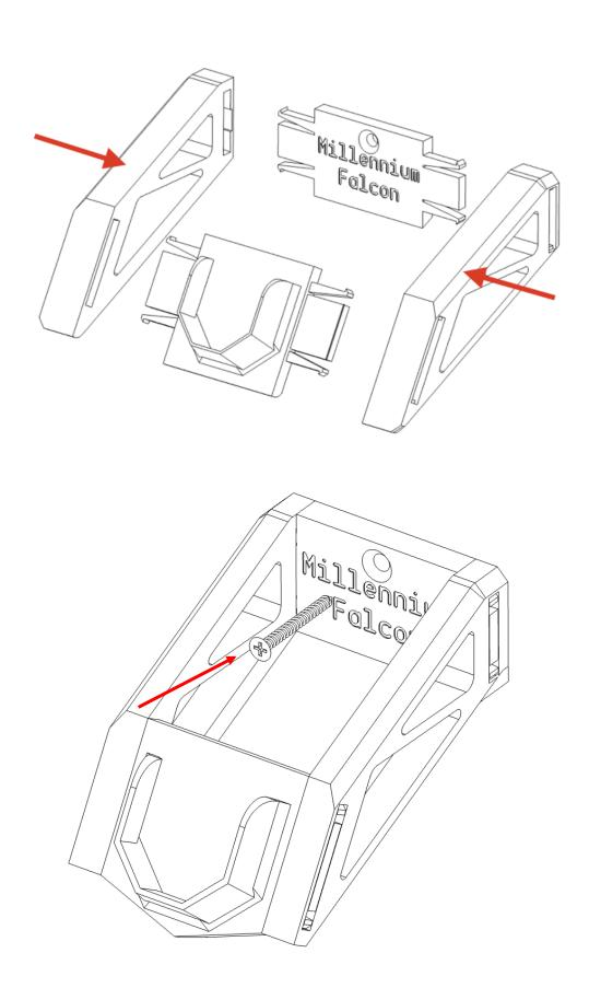
Insert the adaptor piece into the centre of the underside of the ship. Note you will need to remove the turret and ball joint element for the 75257 falcon variant. \*Technic pin from the spare 75257 pieces.
