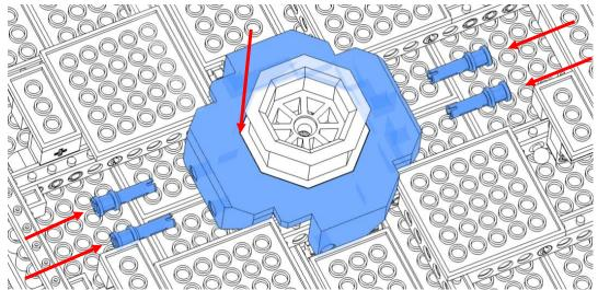
Use the two pins removed previously plus two pins from the bag in the wall mount kit
