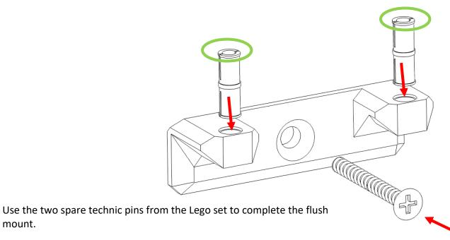
Secure the mount using the included hardware. Do not overtighten the screw (use a screw driver to tighten)
