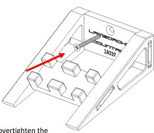
Secure the mount using the included hardware. Do not overtighten the screw (use a screw driver to tighten)
