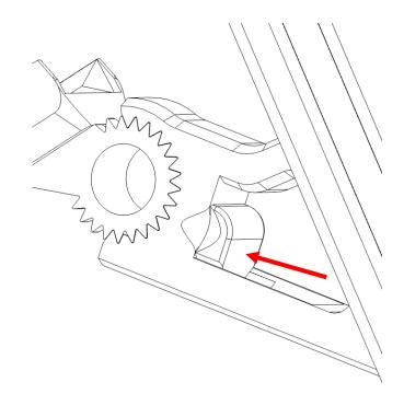
Lock the adaptor in place with the sliding clip
