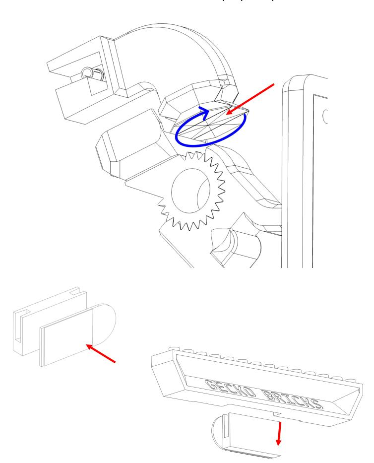
Attach the Minifigure mount lug to the wall first
