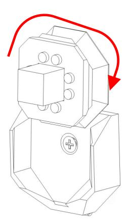
Adaptor piece can be rotated 45 degrees and slide into place in 8 directions.
