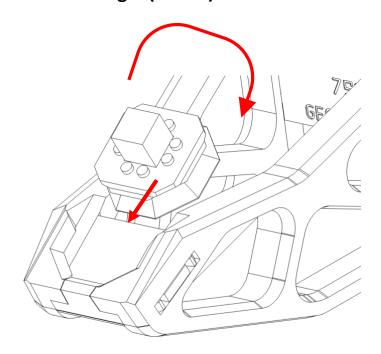
Mount the adaptor piece under the set at the centre of balance.
