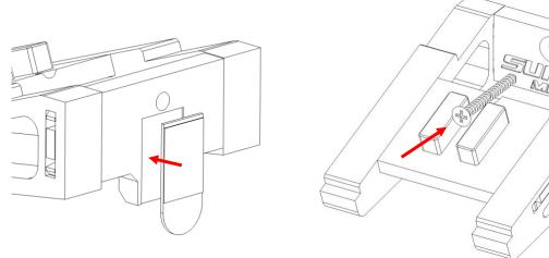
Install both screws into the back stretcher. Do not over tighten (use a screwdriver).
