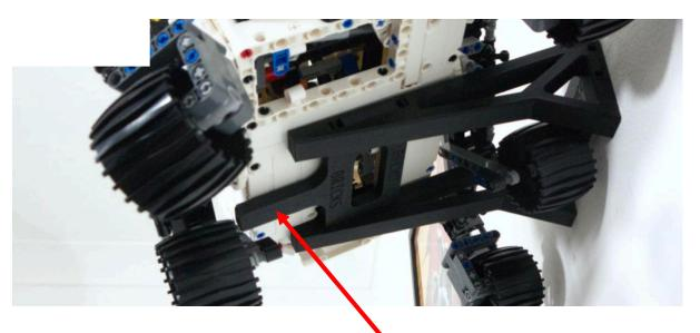
Locate the mounting ledge into the frame of the vehicle. Can be mounted facing left or right.
