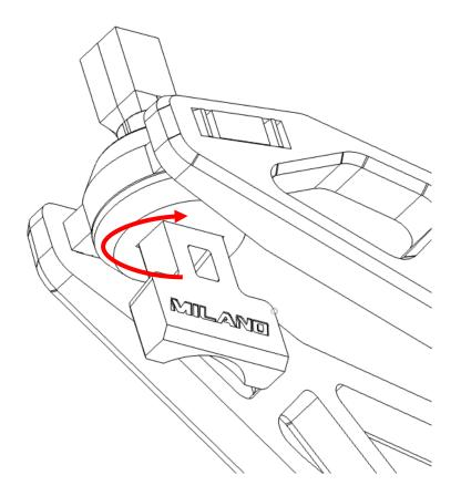
Use the key piece to tighten the ball joint to lock the ship in position.
