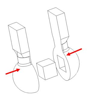
Feed the ball joint through the lower stretcher and screw the ball joint cap on to secure it in place.
