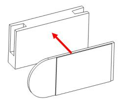
Apply the small 3M poster command strip to the minifigure cleat as shown. Then adhere the cleat to the wall holding in place for 30 seconds.
